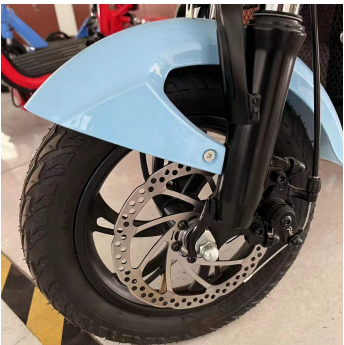
Front wheels and disc brake
