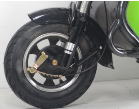
front drum brake Hydraulic Shake
