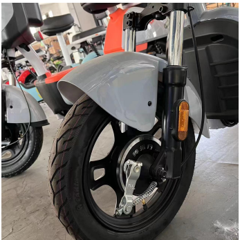
Front wheels and drum brake
