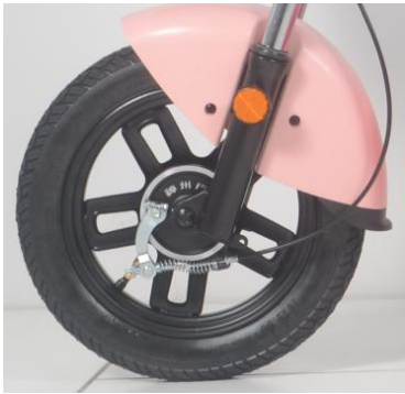
Front wheels and drum brake
