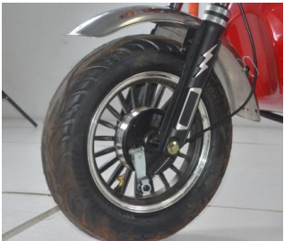
3.00-10 Vacuum Tire Aluminium Alloy Hub
