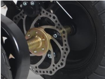
Front and rear disc brake
