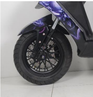
front dsic brake Hydraulic Shake
