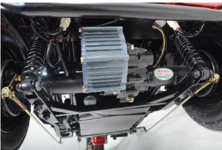
Good quality motor, differential mechanism
