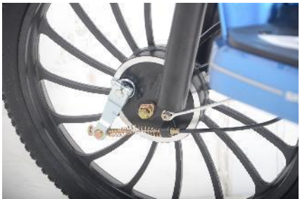
Front Wheels and drum brake
