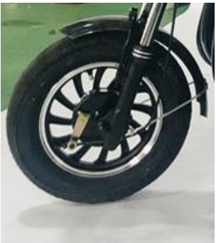
front drum brake Hydraulic Shake
