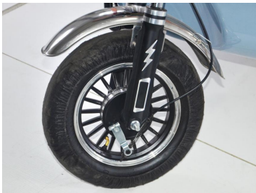
3.00-10 Vacuum Tire Aluminium Alloy Hub
