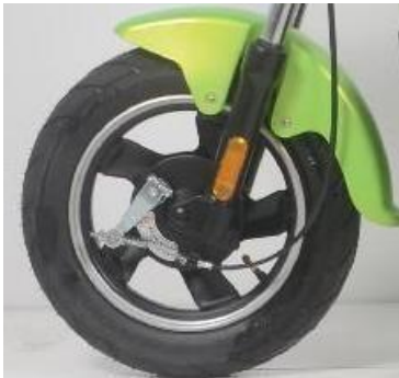
Front wheels and drum brake
