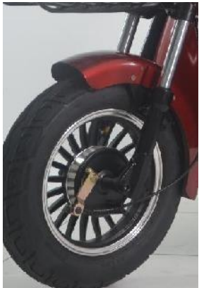
front drum brake Hydraulic Shake
