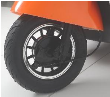
front drum brake Hydraulic Shake
