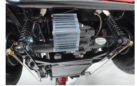
Good quality motor, differential mechanism
