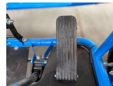
Foot brake one drag two hydraulic disc brake
