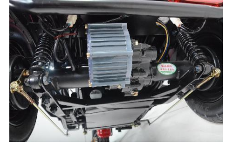
Good quality motor, differential mechanism
