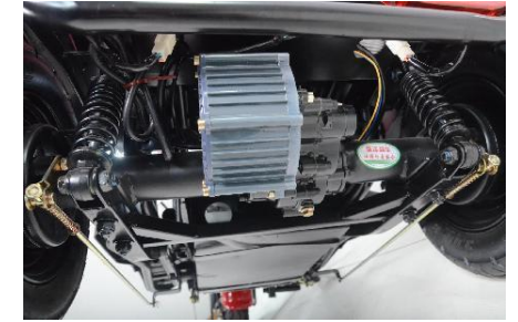
Good quality motor, differential mechanism
