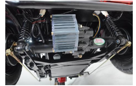
Good quality motor, differential mechanism
