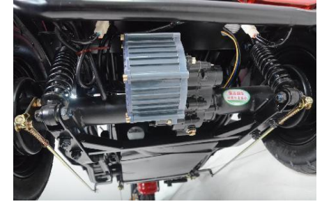
Good quality motor, differential mechanism
