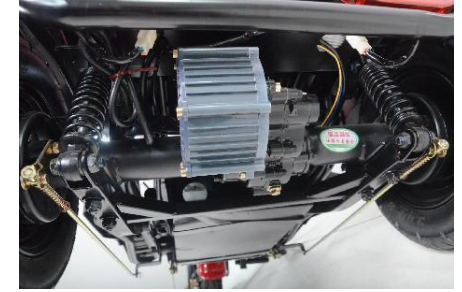
Good quality motor, differential mechanism
