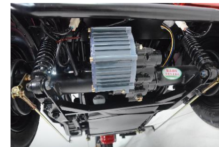
Good quality motor, differential mechanism
